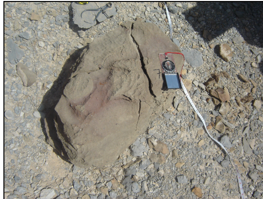
Figure 4. Measuring the orientation, width and length of cracks of clasts (source: author).
